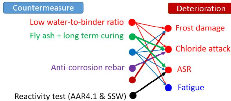
Fig. 4 Multiple defense system applied to bridge deck (Mukai Sadanai Bridge)
