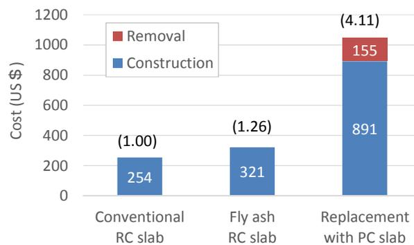
Fig. 4 Cost of conventional and fly ash RC slabs (Mukai Sadanai Bridge)
